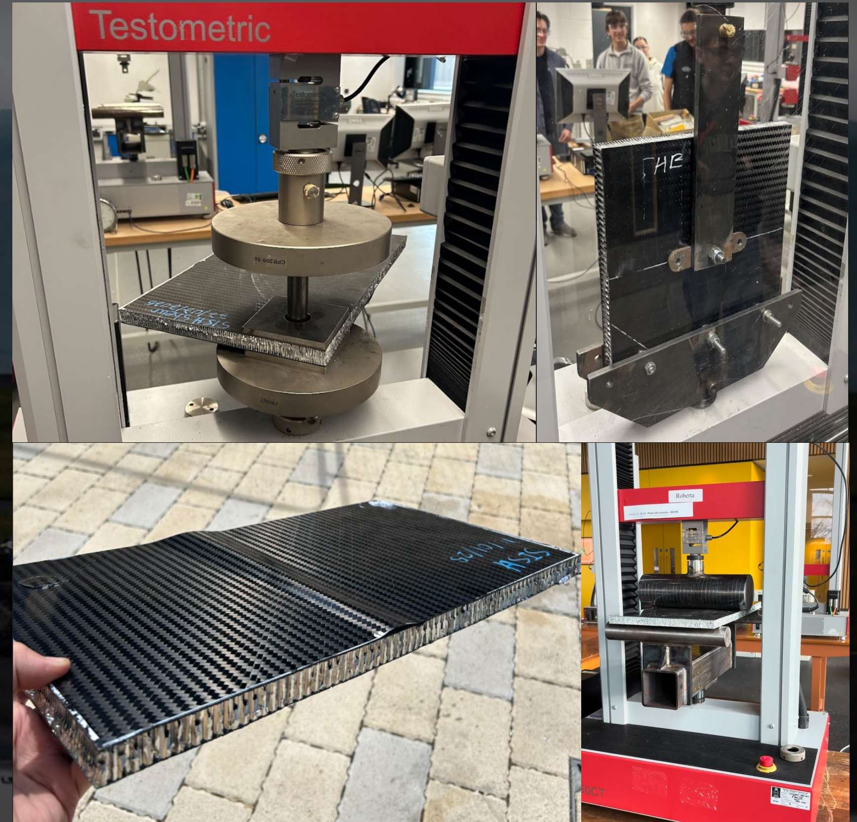
Shear testing (top left), tear out testing (top right), skin buckling (bottom left), and 3PB testing (bottom right)
