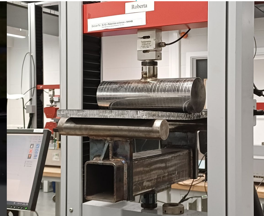
3PB model and real-world test.
