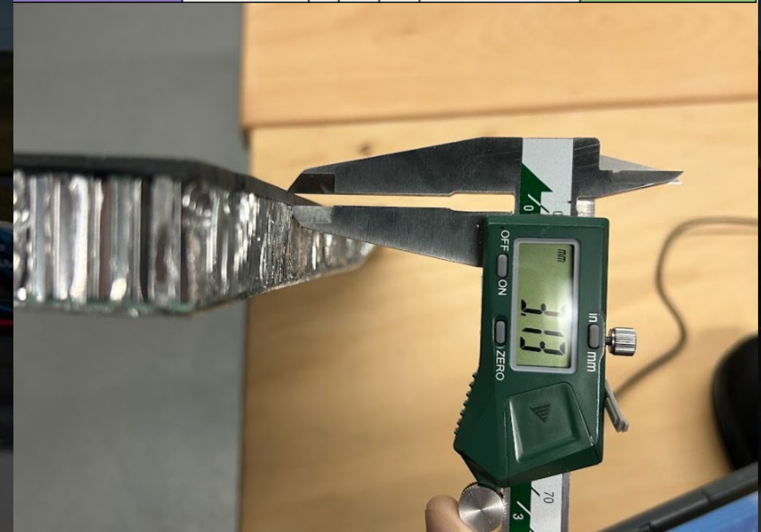
Proof of fibre directions <50% and the differences in skin thickness of the front bulkhead.
